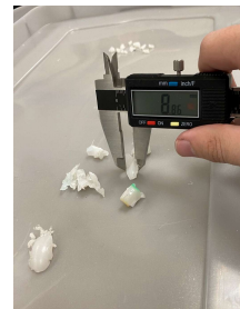
Figure 4: Testing shredded parts
