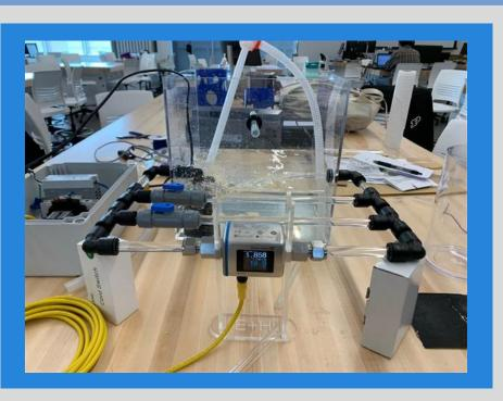
The testing phase of the project consisted of operating the system and checking for leaks with the seals, tubing, and fittings. The three primary sensors were checked for proper connection and operation.
