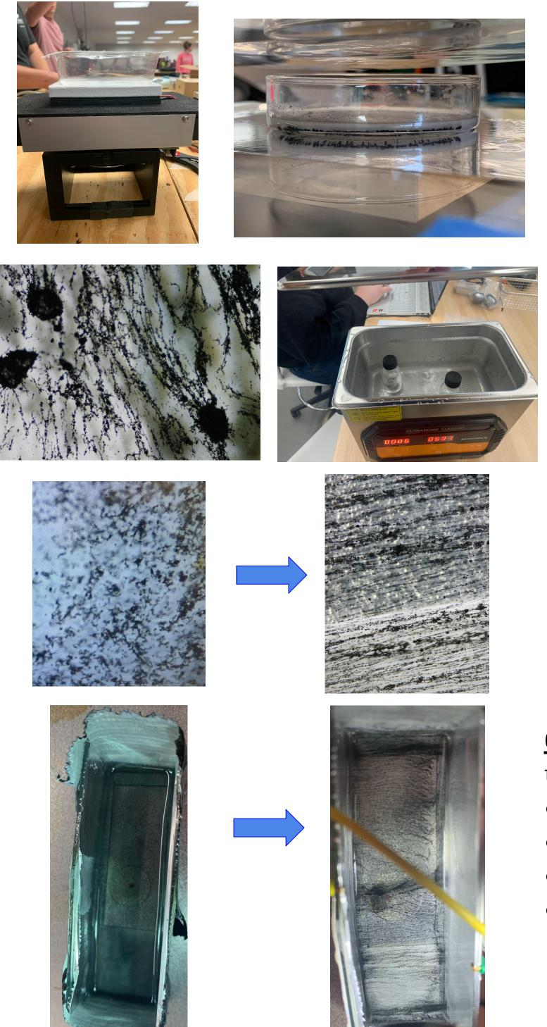
Solution Creation: Suspend CNTs within a state-changing material so that we can capture them in a rigid form
