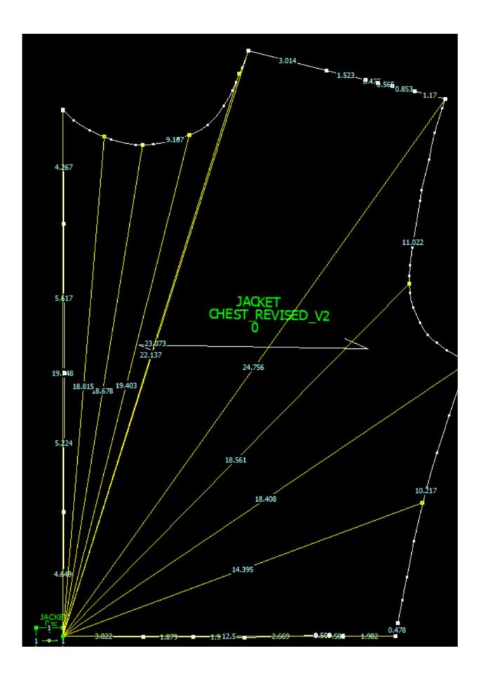
Our final design focused on digitizing eleven key jacket components using a fixed coordinate system to ensure geometric accuracy. Patterns were photographed and traced in TUKAdesign using the Virtual Digitizer and screen calibration tools.
