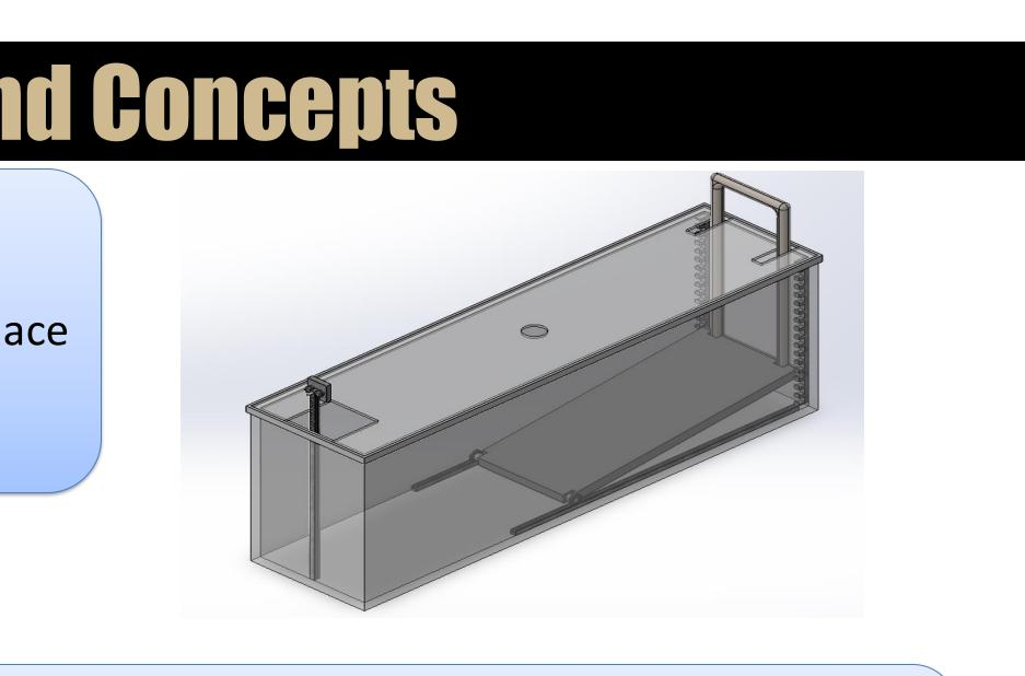
A new method of wave generation was ideated. This concept pushes water columns uniformly instead of creating ripples. This would create more uniform waves.
