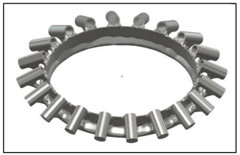
Fig. 2 – Generative Design of "Rotor Ring"
