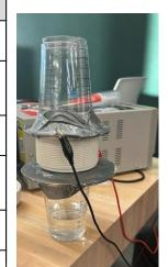
The final design we built utilized a drip filtration method of slowly letting the water drip through the filter under no pressure while being subjected to a constant low voltage parallel to the flow of water, and thus creating an EMF that repelled the charged salt ions.
