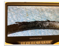
Backup Seal after 10,000-cycle test under microscope
