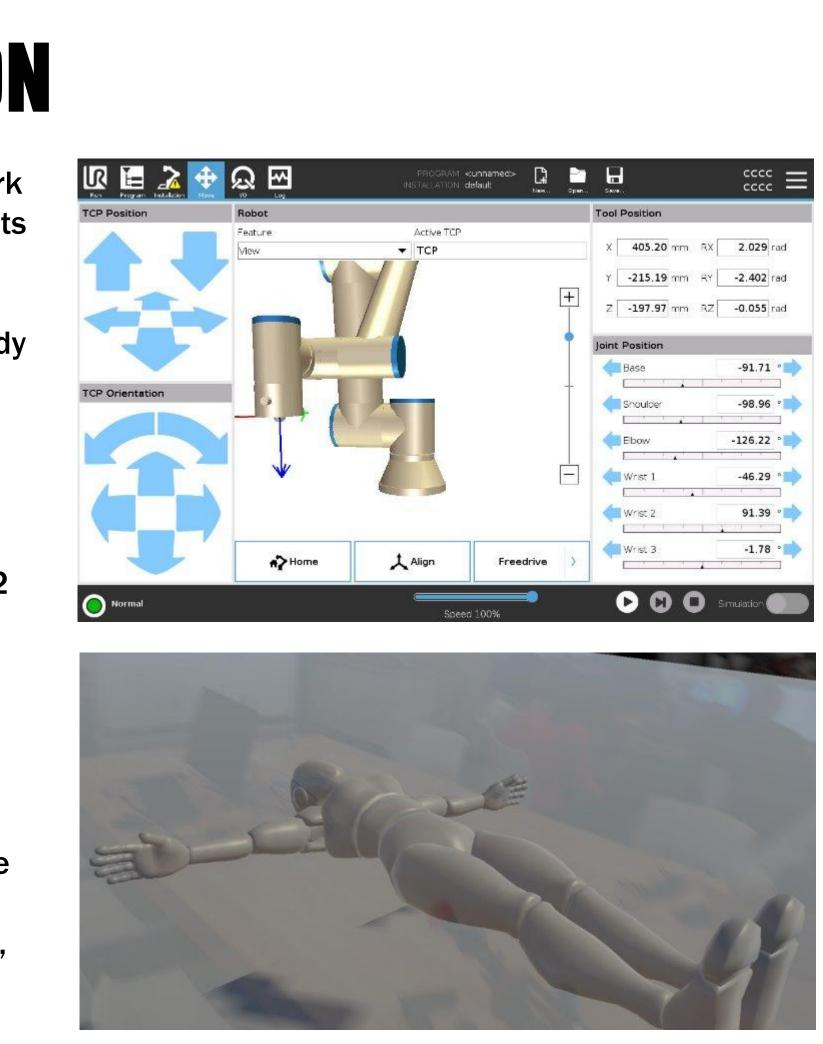
Our most successful prototype was the VR simulation in Unity with the HoloLens2. This consists of a of the surrounding area and a virtual 3D representation of a human body that can be further augmented to simulate an evidence collection procedure. The merits of this system include the immersion and the ability to add instructional material into the program to help reinforce the user's training.
