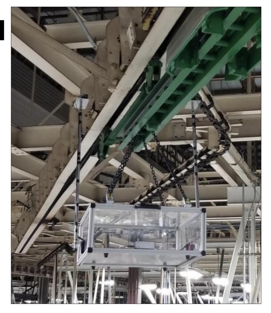
When tested, our product worked a little differently as expected. Our cameras were not able to take the most optimal photos due to the servos being loose, causing the arms to be in lower angles. The camera was also too sensitive when detecting cracks. The LIDAR sensors worked well when objects were detected. The battery life was better than expected, but there were some power draw issues related to the Arduino.
