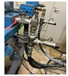
Hydraulic Pressure Sensors 3 T-fittings and adapters for sensors
