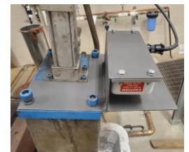
Position/Velocity Sensor Bracket made of 1/8" steel flat stock
