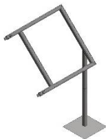
Control Box Frame Built from 1/8" steel box tube
