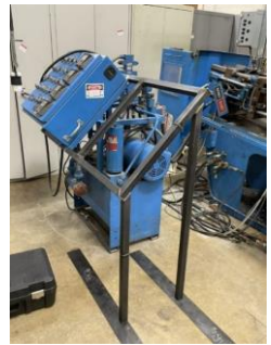
Control Box Frame Built from 1/8" steel box tube
