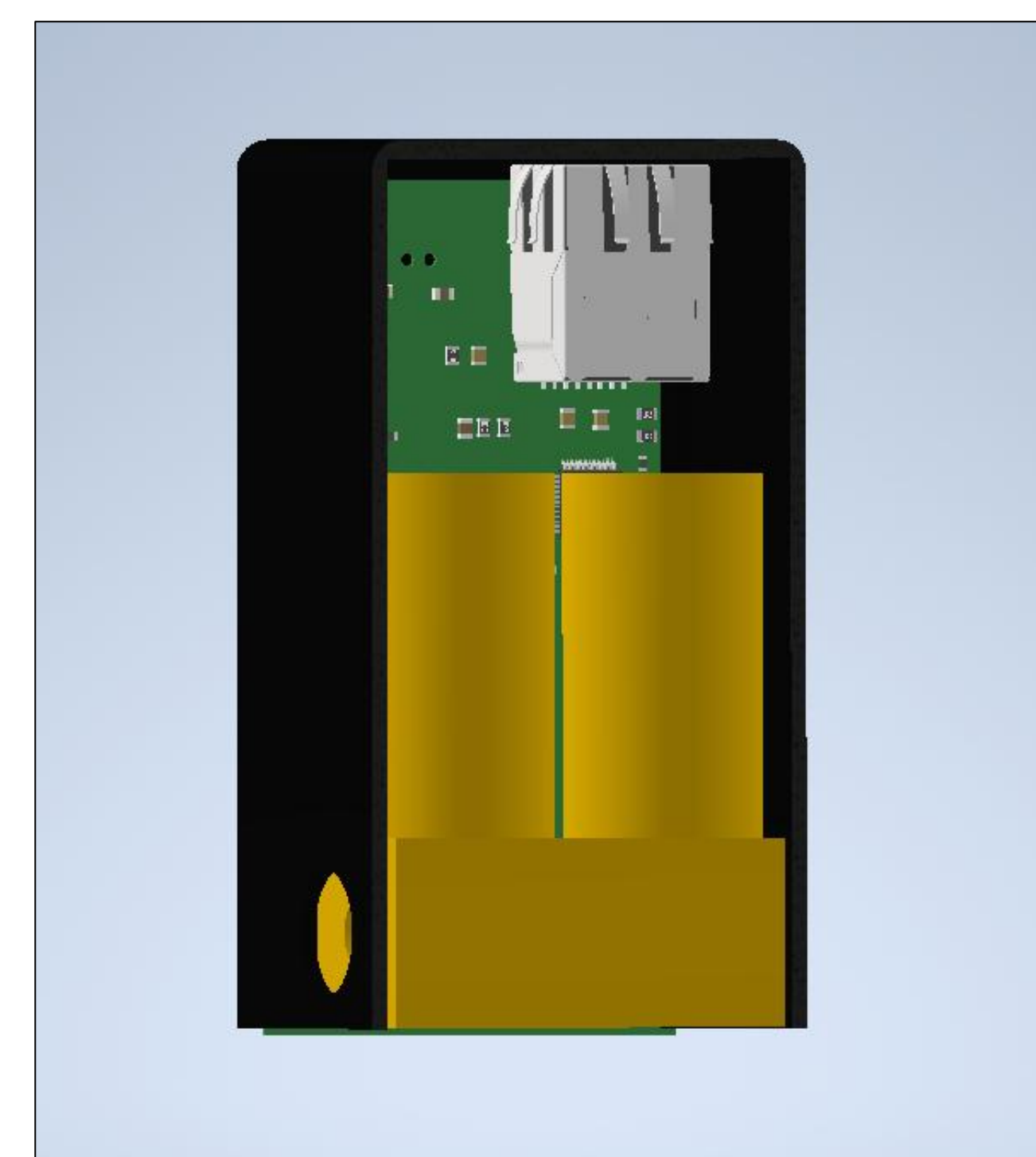
3D rendering of the valve construction with PCB
