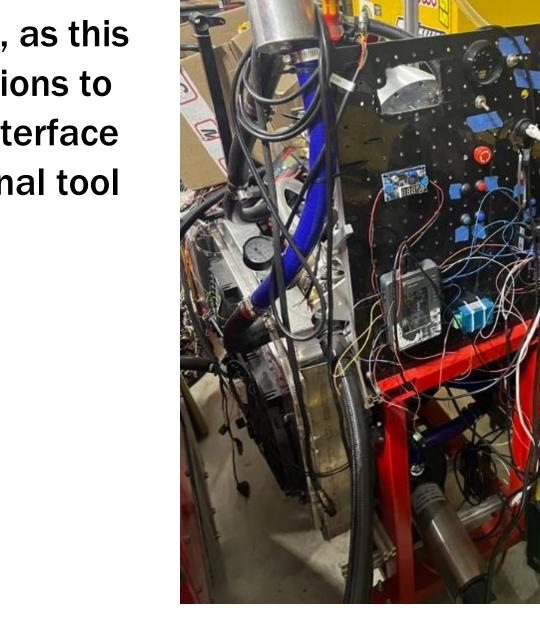
A previous solution for the dyno control included using a TI myRIO. This required many different devices wired to the primary device in order for this to function. There was also no interface with the CAN bus for communication with the engine ECU, which made user input difficult with two different software packages as well as added sensors for closed-loop control.
