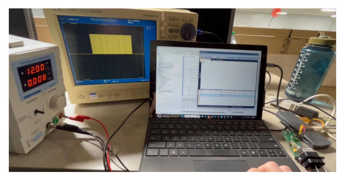
Unfortunately, the Purdue Formula SAE team was not prepared for dyno operation so only bench testing was used to prove functionality. CAN messages between engine ECU and controller were simulated via PCAN to control stepper output. Oscilloscope was used to verify appropriate response from controller.
