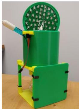
Final 3D printed casing design
