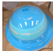
Figure 2. Fiberglass Endcap Mold
