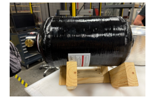
Figure 12. Reference Model Water Tank for Testing
