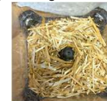
Fig. 5. Insufficiently ground grass. This example was ground in a blender which was incapable of grinding to the desired size.
