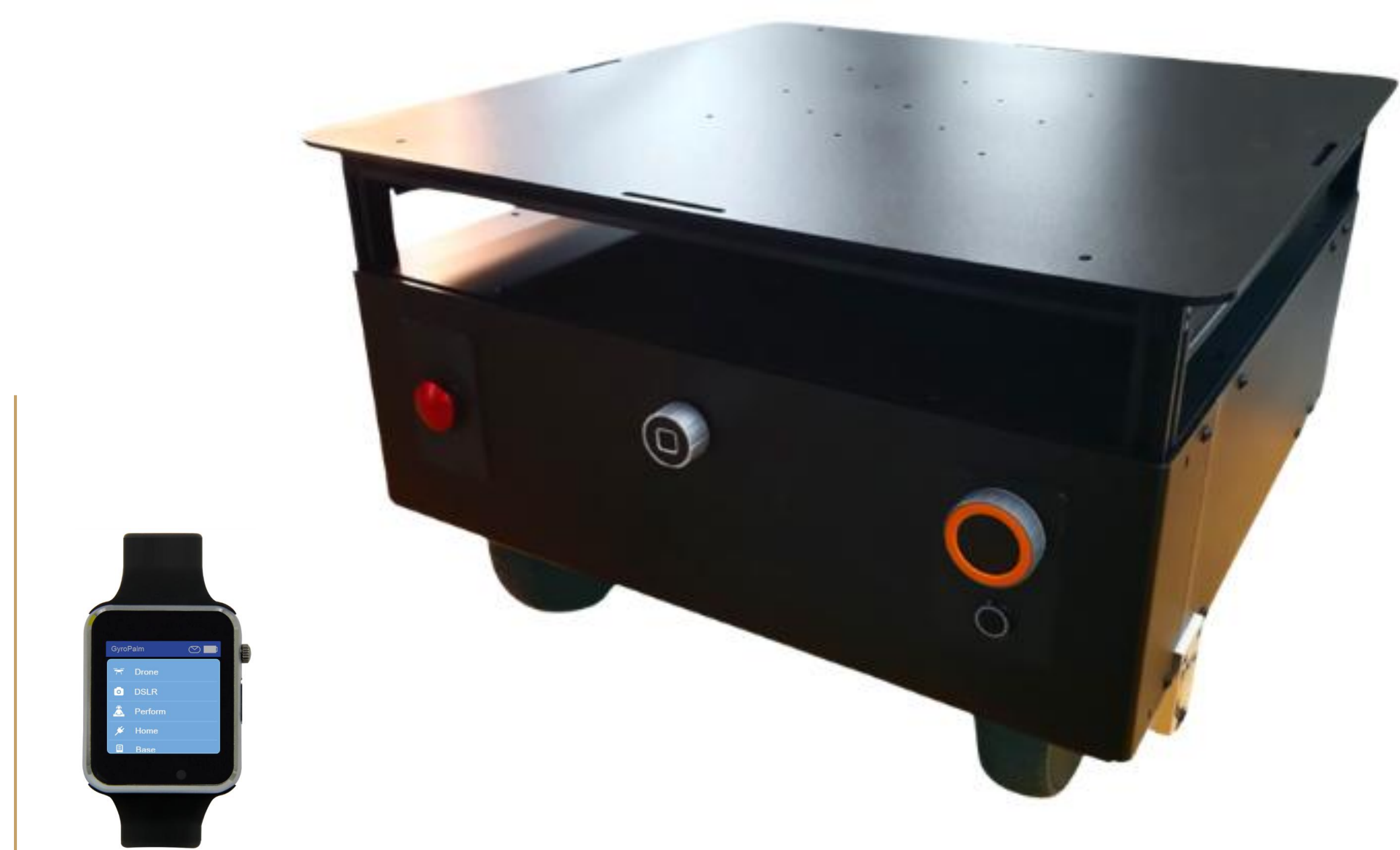
Gyropalm Omnibot V2 and Gyropalm Encore Wearable communicating wirelessly through ESP-NOW or Teleop
