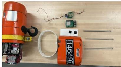
The final design implemented the factors identified in the design requirements. The Raspberry Pi was capable of measuring orientation, acceleration, and temperature with the use of the SenseHAT peripheral device.
