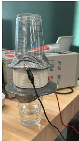
The final design we built utilized a drip filtration method of slowly letting the water drip through the filter under no pressure while being subjected to a constant low voltage parallel to the flow of water, and thus creating an EMF that repelled the charged salt ions.
