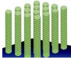
The initial designs were based around using aligned nanotubes with diameters large enough for water but smaller than salt and forcing water through
