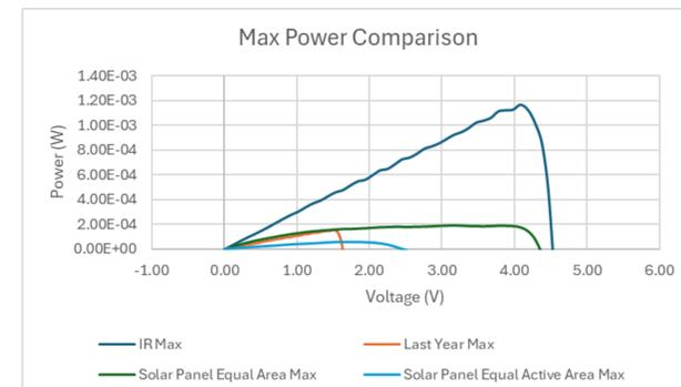
Figure 16: Max Power Comparison of Array vs. Solar Panel
