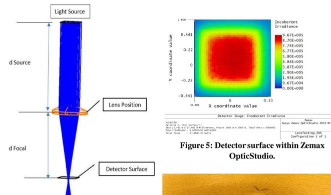
Figure 4: Zemax OpticStudio testing layout with labeled features.
