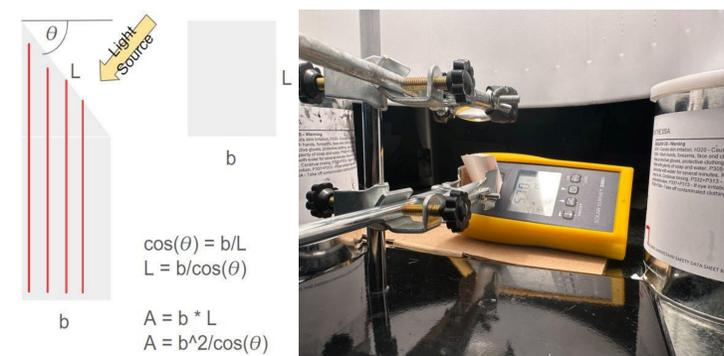
Figure 10 & 11: Testing setup for surface area tests
