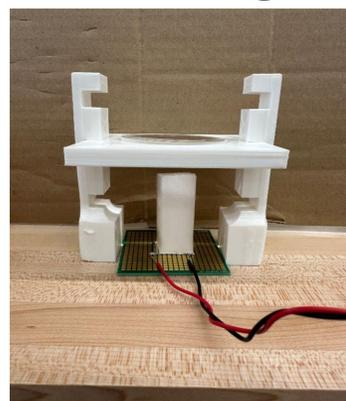
Figure 9: The lens, 3D Geometry, and LED array all held together by a printed holder
