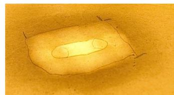
Figure 6: The outlined concentration area and illuminated area during focal point adjustment tests.
