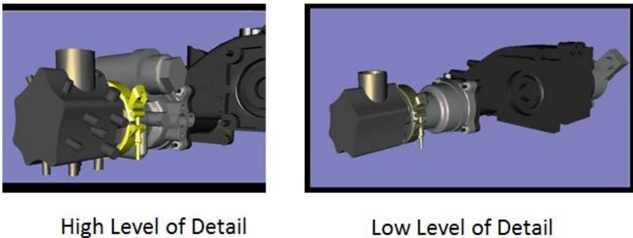
Fig. 4. Fuel Pump and Gear Box from F-109 Engine. Comparing High and Low Levels of Detail and Interactivity of the CAD Assembly Work Instructions.
