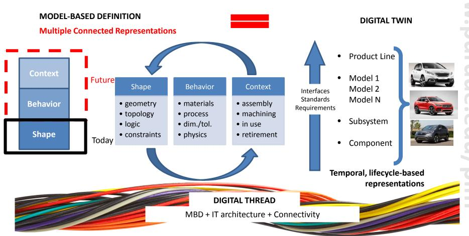
By comparing digital product data to the physical performance of the object, variation can be tracked and used to inform design of next-generation products, develop predictive modeling and validation schemes for products, and to diagnose and solve problems that occur.
