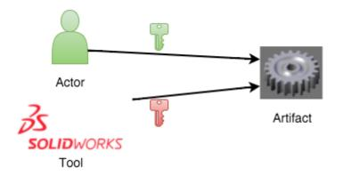
The Actor cryptographically signs the artifact with a personal key The Tool cryptographically signs the artifact with a version-specific key This cryptographically guarantees the 'who' and the 'how'
