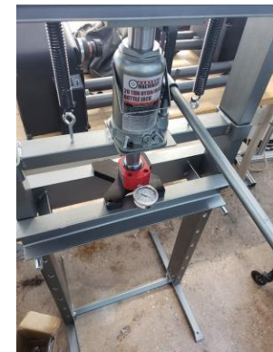
Testing load cell
